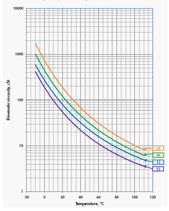
Viscosity - Temperature Diagram for Shell Tellus S4 ME
